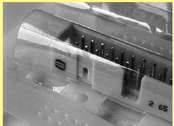
SEK connector mounted in a tape ready for placement using an odd form assembly station.
