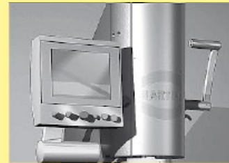
Visual guiding system via touch monitor
