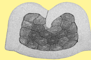
B shape cross section stamped contact
